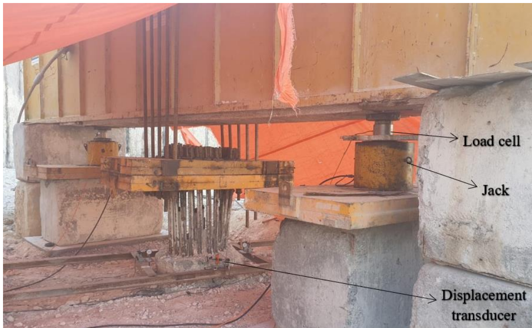
Fig.1. Traditional pull-out test set up
